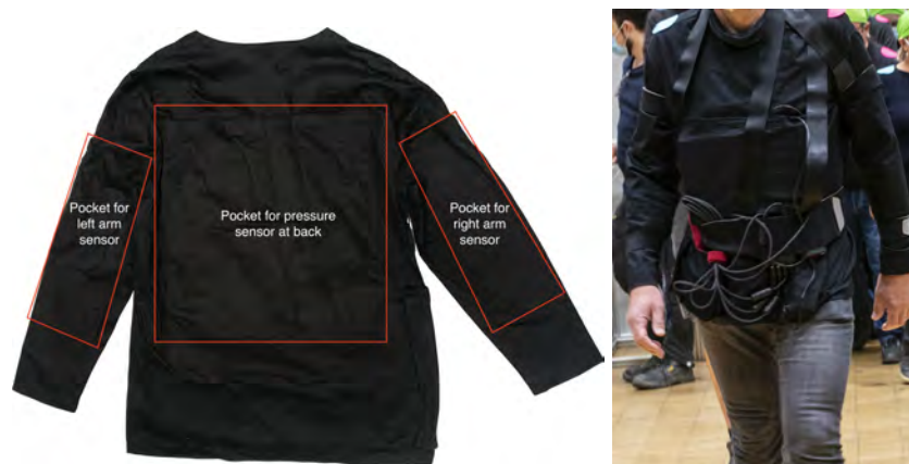
Figure 16 Wearable T-shirts with pockets for the pressure sensors. a) Back view of the T-shirt. Pressure sensors can be stored in the pockets for the left arm, right arm and the back. b) Participant during an experiment. The tablet is stored in the chest pocket.
