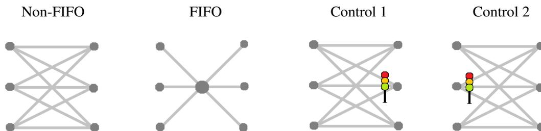
**Figure 1** Illustrative scheme for the four types of intersection: Non-FIFO (optimal), FIFO, and the two regulated models with control on the incoming roads and on the outgoing roads, respectively.
