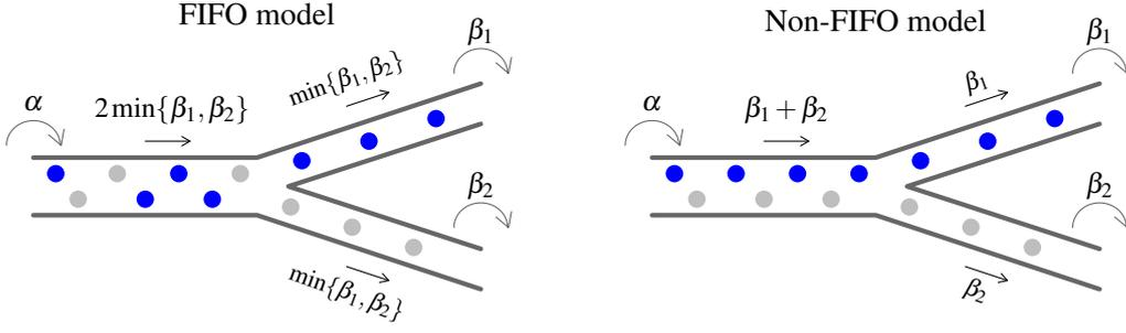
**Figure 3** Illustrative comparison for FIFO and non-FIFO models on a  $1 \times 2$  diverging intersection with  $p = (0.5, 0.5)$  and  $\alpha \geq 2\min\{\beta_1, \beta_2\}$  (FIFO model, left panel) or  $\alpha \geq \beta_1 + \beta_2$  (non-FIFO model, right panel).
