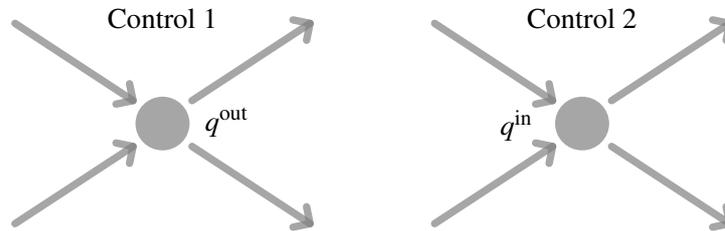
**Figure 4** Illustrative scheme for the first signalized model Eq. 10 for which the control operates on the outgoing roads (left panel) and for the second signalized model Eq. 11 for which the regulation operates on the incoming roads (right panel).
