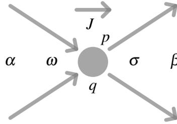
**Figure 2** Notations for a point-wise intersection.  $\alpha$  and  $\beta$  are the demand upstream and the supply downstream;  $\omega$  and  $\sigma$  are the flows on the incoming roads and on the outgoing roads;  $p$  is the assignment of the demand by direction (route choice);  $q$  are some priority rules;  $J$  is the total flow.
