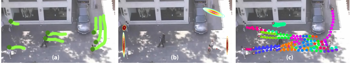
Figure 2 Pedestrian Movement Dynamics Learning: A one-frame example: (a) input consists of pedestrian trajectories (green) from the video; (b) probabilistic distributions of entry points at one frame computed using the Gaussian Mixture Model (shown as elliptical regions); and (c) movement flows grouped by the characteristics of pedestrian dynamics, in which each grouping is represented by the same color.
