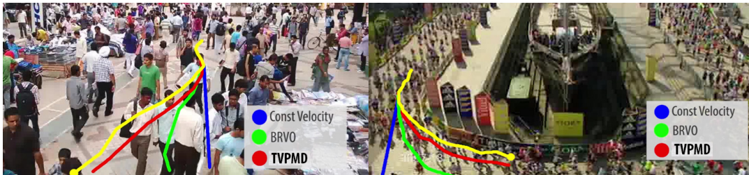
Figure 7 Pedestrian Prediction Results: We demonstrate the improved accuracy of our pedestrian path prediction algorithm using TVPMD over prior real-time prediction algorithms (BRVO, Const Vel) and compare them with the ground truth (in yellow). We observe upto 12% improvement in accuracy.
